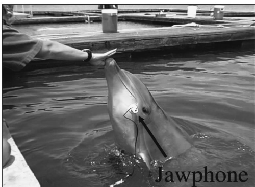
FIG. 5. The jawphone positioned over the dolphin's left pan bone or "acoustic window."
