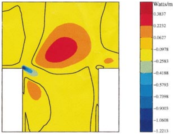
FIG. 7. Acoustic source power time averaged over the acoustic cycle for St=0.4 , u'/U=0.5 (black lines denote zero amplitude).
